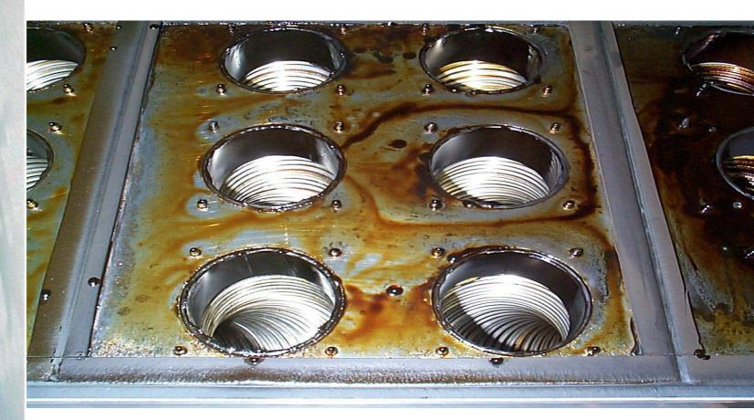
The same condenser tube after self-cleaning cycle flux is re-liquified and drips into collector trays
